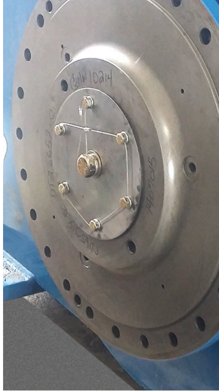
Figure 4: Flange Retainer with Safety Wire
